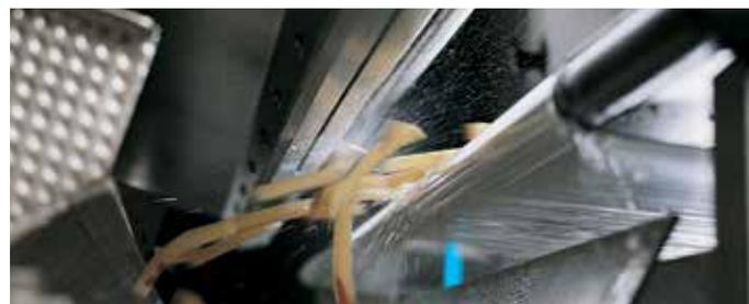
The product then arrives in the inspection zone where six cameras detect defects from all sides. The position of the product that does not meet these quality standards is recorded in the electronics. This information is passed on to the manifold (positioned at the end of the conveyor belt) where the right air gun removes the affected French fries just a few milliseconds after detection, while the good product continues untouched into the accept chute and on to the production line."
