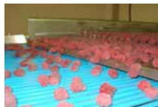
Infeed of IQF raspberries on the Primus™ equipped with O-ring belts.
