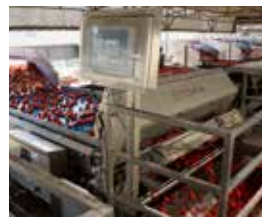
Sentinel II sorting pre-peeled tomatoes at high capacity.
